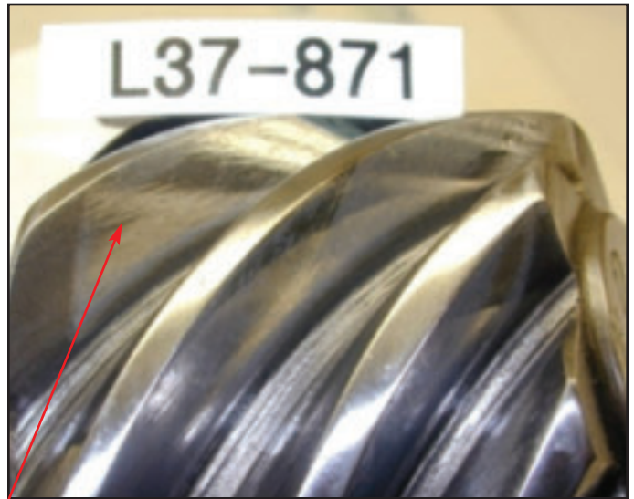
Pinion gear - original machine marks still present.
