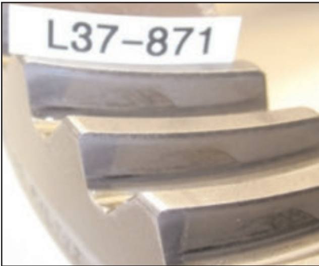
Ring gear exhibits very low wear.
